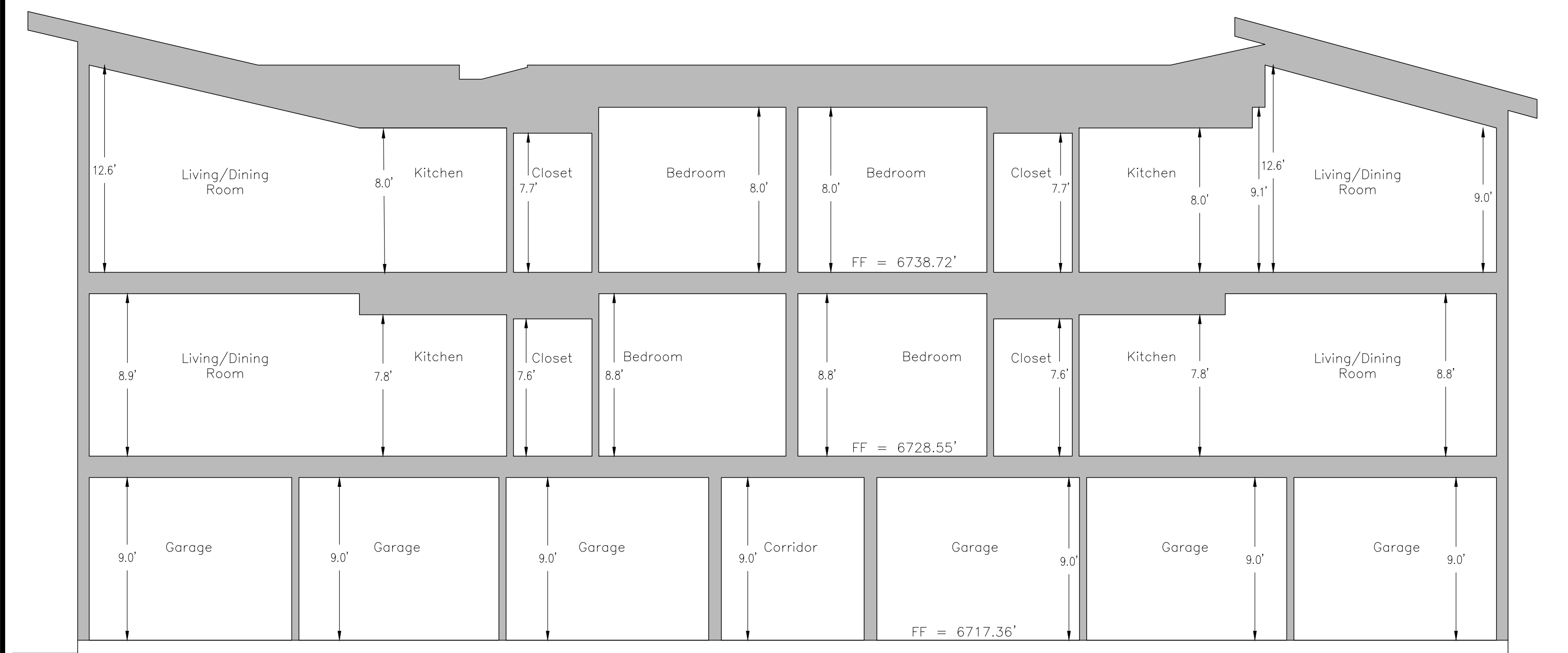
Building A Cross Section 2 Facing Northeast
