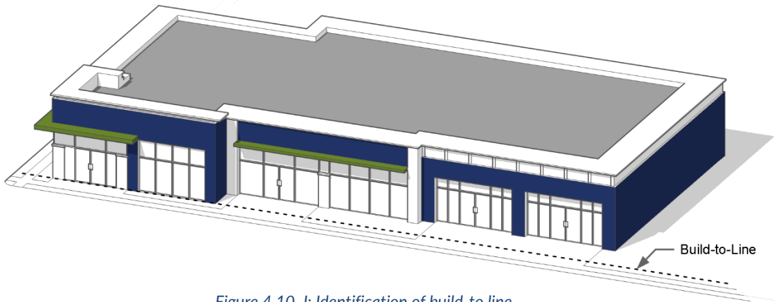
Figure 4.10-J: Identification of build-to line
