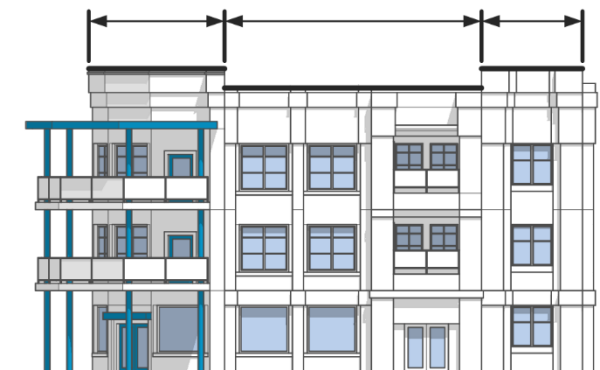
Figure 10-C: Roof line change example
