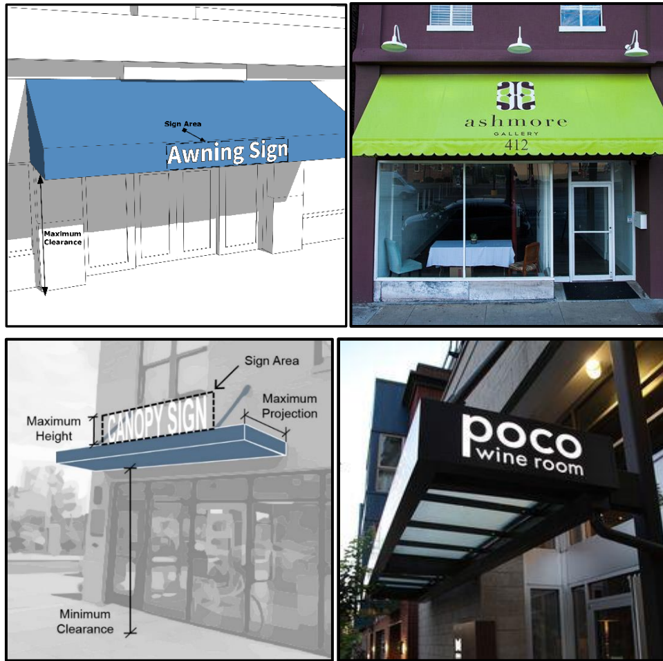
Figure 4.16-A: Awning and Canopy sign detail
