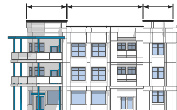
Figure 10-C: Roof line change example
