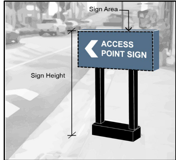
Fig. 4.08-E: Access point sign
