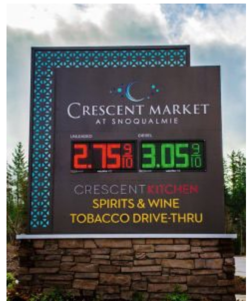
Fig. 4.08-I: Example EMD that is approximately 12% of the sign area, not including the base.
